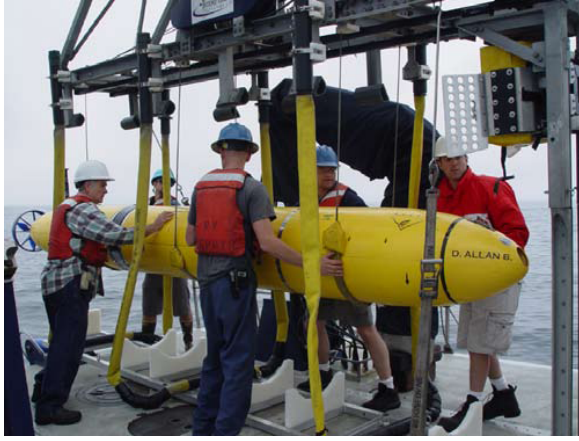
Fig. 4. MBARI Dorado class mapping AUV being prepared for deployment via an over-the-stern J-frame crane [7].
